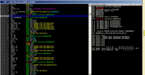
First, a call to 0×00402225 is made (main function of the shellcode), where we can see a pointer to "calc.exe" getting pushed onto the stack, and WinExec being located
