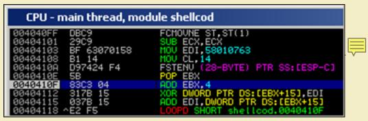
Again, the XOR instruction will produce the original bytes and write them at EBX+15. Next, the result is added to EDI (which is used to XOR the next bytes in the next iteration) ...
